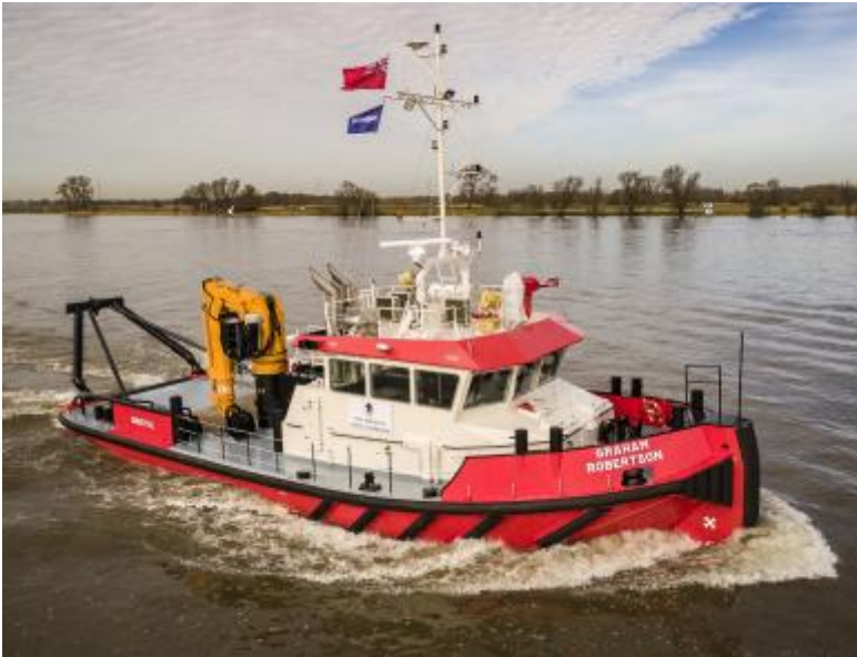
Survey & Plough Dredger 'Graham Robertson'
